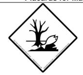
Packages and cargo transport units containing dangerous substances which are classified by the IMDG Code as "marine pollutants", must have the markings shown here, which must be durable. They must be placed close to the risk labels or risk placards of the goods. The dimensions of the marine pollutant markings must be a minimum of 10 cm per side for packages and 25 cm per side for cargo transport units.
